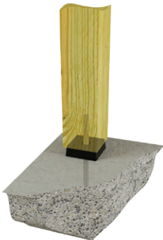
Typical CPB installation
